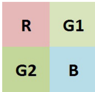
Figure 1. Basic 2 by 2 pixel Bayer filter block of a Canon DSLR. Other brands may use a different order of colours. The two green filters have the same spectral transmission characteristics.
