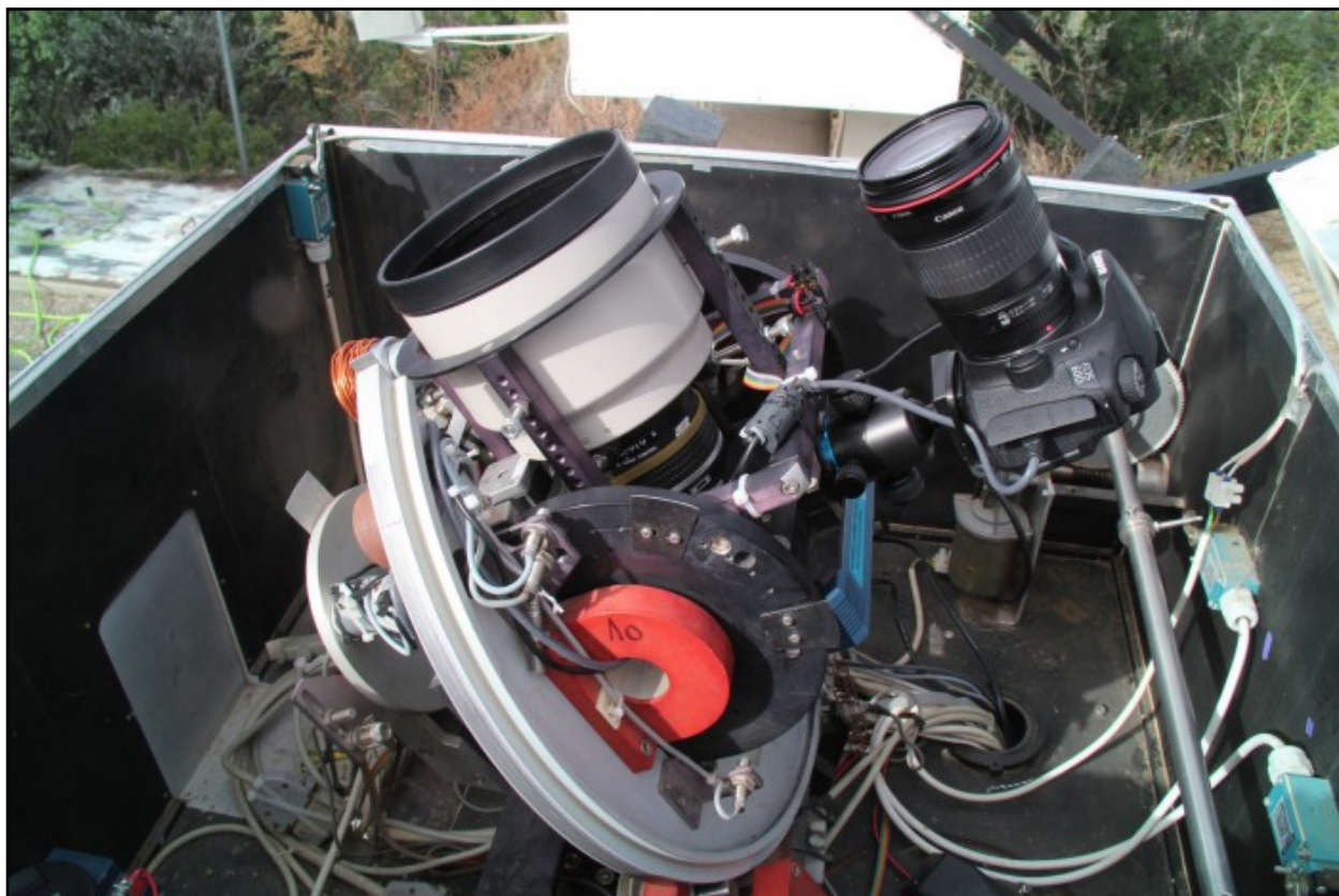
A Canon EOS 60D DSLR camera attached to HAT 10, one of the telescope units making up the HATNet (Hungarian Automated Telescope Network). For details see the paper by Zhang et al referenced in Publication Watch on page 12.
