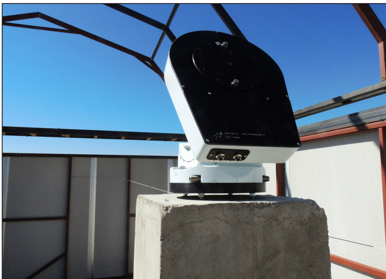
The base of the MI500/750F mounted on its column March 2016.
