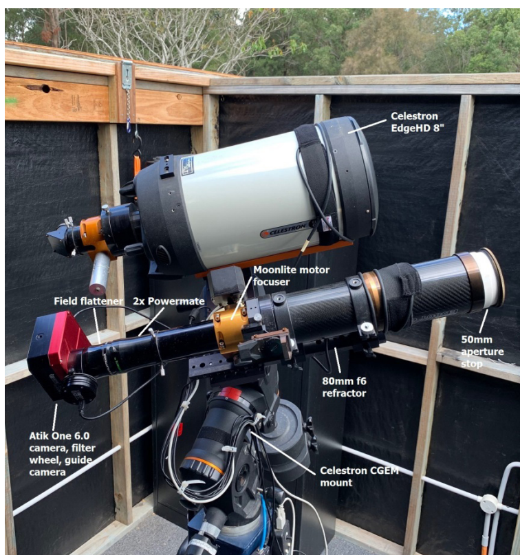
Figure 1. Photometry setup used for imaging eta Carinae.
