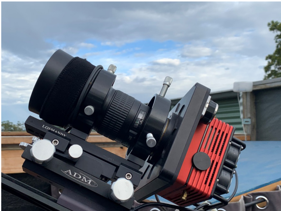
Figure 3. 200mm f2.8 camera lens and SBIG STT3200-ME CCD camera.
