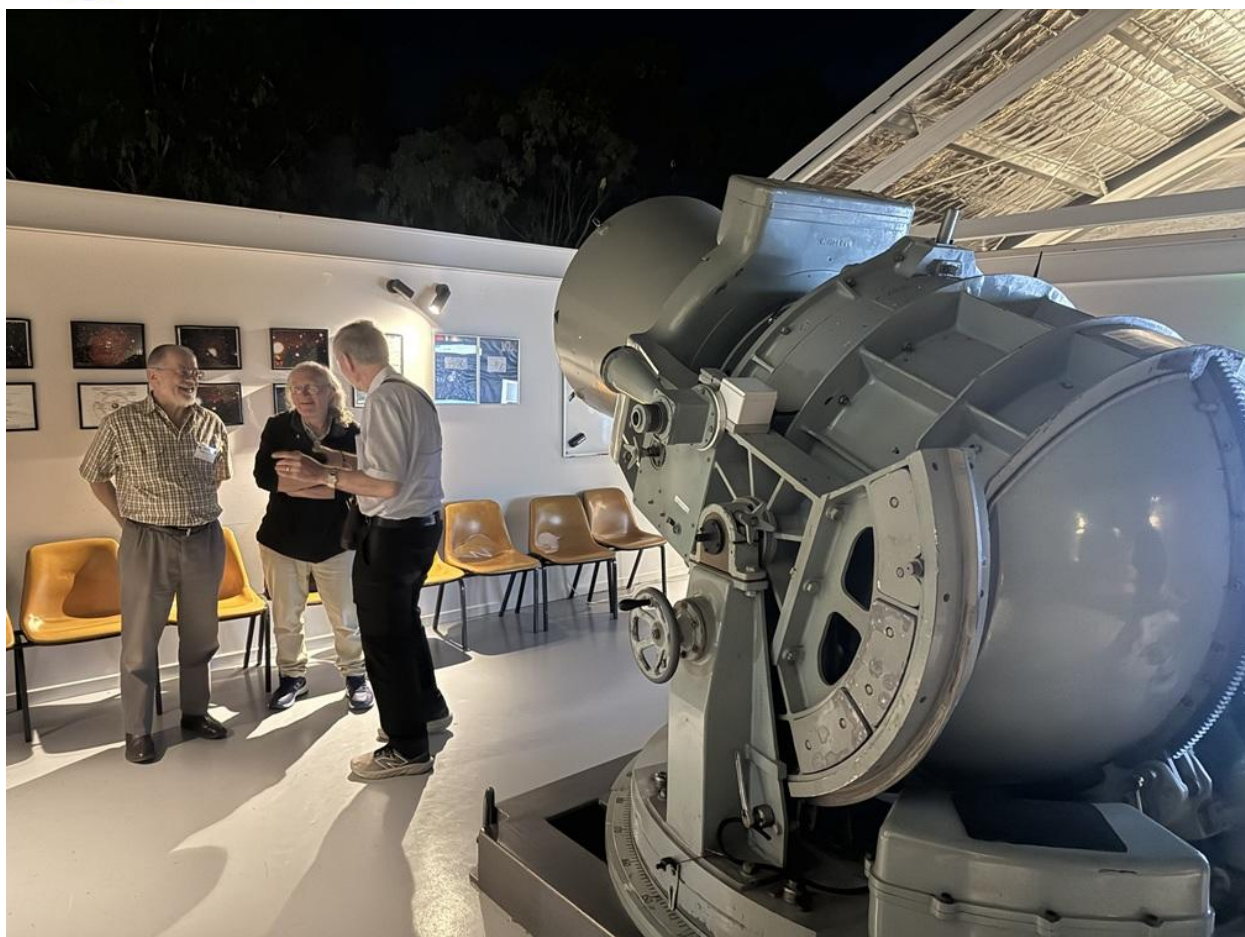
The historic 34-inch Hewitt Camera at the Tamworth Regional Astronomy Club Inc (TRAC). Originally built in the 1950's for tracking 'Blue Streak,' a British ballistic missile, then relocated to Siding Spring to monitor artificial satellites (1982-1990). Purchased by TRAC in 2016 and refurbished, including replacing the plate camera with a CCD. Now used for public viewing.
